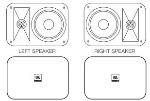
**Note:** Be sure to rotate the JBL grille badge 90 degrees if you are mounting these speakers in the horizontal position. Simply remove the grille, push the badge from the inside and rotate it accordingly.
